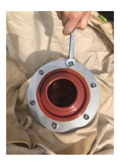
• Push one piece of your flue pipe into the silicone using washing up liquid or other lubricant to help it slide through. This is because it's quite stiff and tricky to do after the tent has been erected.
